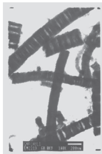
Figure 3 TEM image of the segmented carbon nanofibers (Reaction temperature 600°C; Reaction time 30 min.; Gas flow rate: C 2 H 2 15 ml/min; and H 2 150 ml/min).
